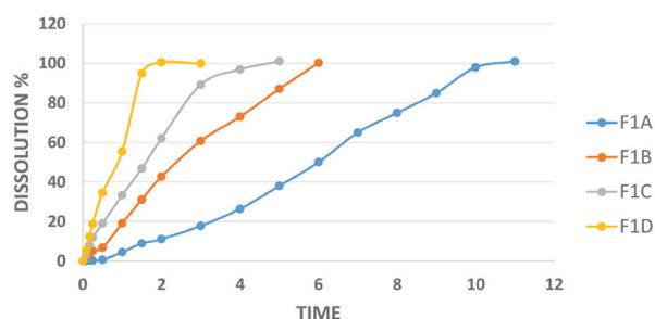
Fig. 2 The dissolution profile of F1 tablets in devices A, B, C, and D.
