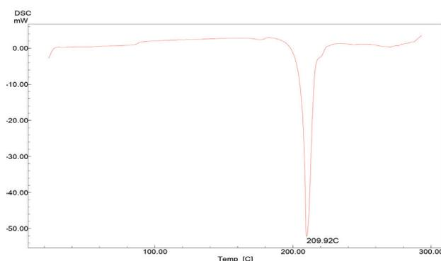
Fig. 6 DSC thermogram of pure baclofen.
