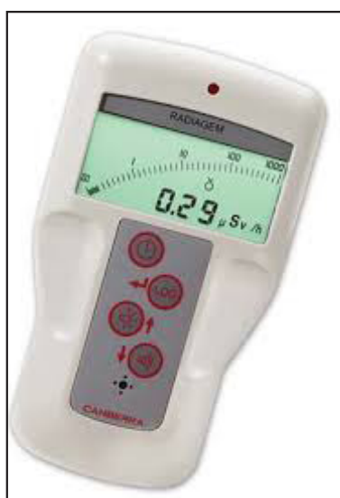
Fig. 3 Survey meter that measures radiation exposure.
