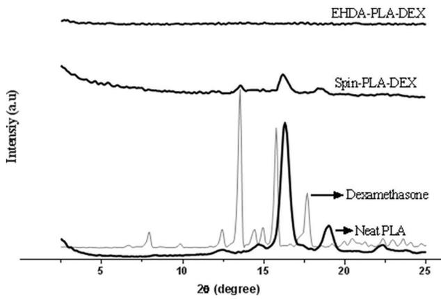
Fig. 1 X-ray diffractograms of neat PLA, dexamethasone, Spin-PLA-DEX and EHDA-PLA-DEX.
