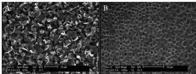
Fig. 2 SEM images of the morphology of coating that show microbead-and-nanofiber structure of EHDA (a) and micro/nanoporous (b) structure of spin coatings.
