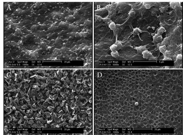
Fig. 6 SEM images of platelet adhesion and activation on EHDA-collagen (a and b), EHDA-PLA-DEX (c) and Spin-PLA (d) samples.
