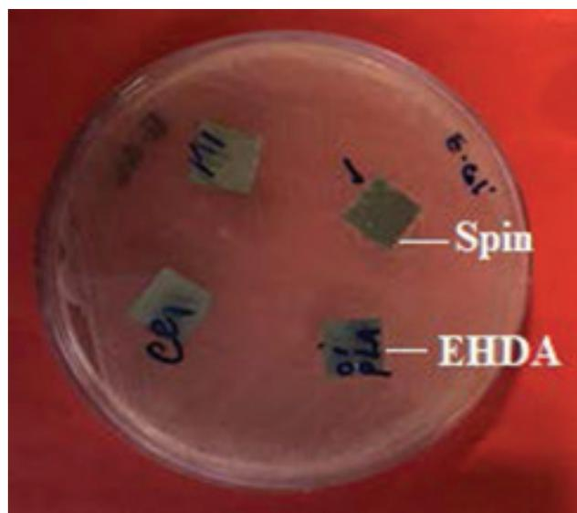
Fig. 9 Agar test of bactericidal effects of coatings.
